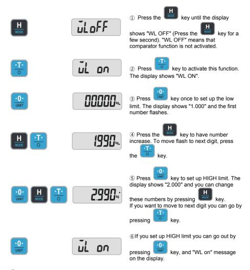
⑦ If you set up HIGH limit and LOW limit incorrectly, "Err" will be shown on the display. Then you may need to set it up again. For example, setting LOW LIMIT=2.990 kg and HIGH LIMIT=1.990 kg this is incorrect setting because HIGH limit is lower than the LOW limit. When HIGH and LOW limit are set as the same or above maximum capacity it still shows "Err" message.
